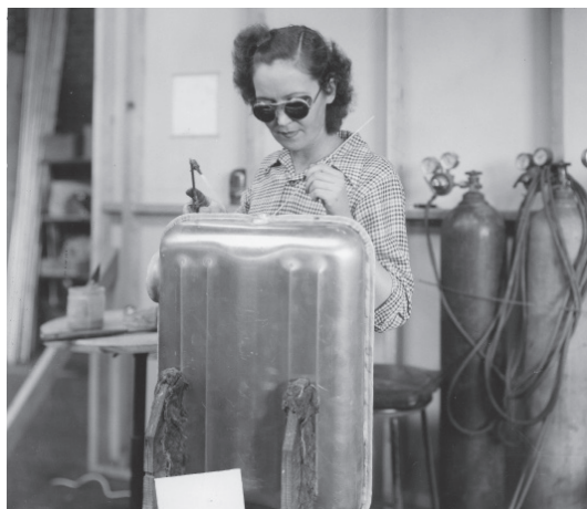
(Below) A woman welding a seam on a fuel tank at the Bellanca Aircraft plant in New Castle.
