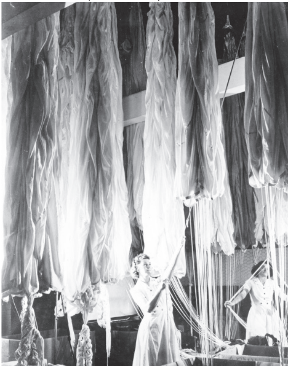
Inspection of DuPont Nylon parachutes after test flight.
